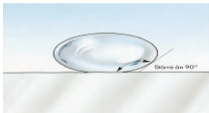
Picture No. 4: Angles of between 90° or more will result in bad adhesive ability
