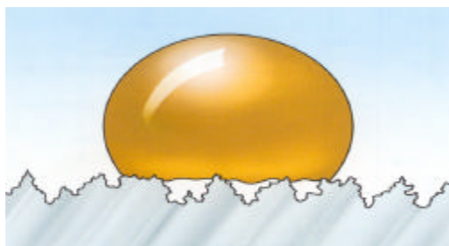
Picture No. 2: When the surface tension of the glue is higher than of the material there is no adhesion since the surface is not wet.
