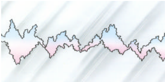
Picture N0.1: Even The most smooth surface has asperity that is several hundred Angstroms ( 1 \text{ \AA} = 10^{-10} \text{ m} ) deep. The picture shows two
